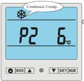
○ Under running status ,press △ and ▽ to check the current status of the unit!You can check water-in/water out temp,condenser temp and ambient temp,please note no motion on the display for 5s,the LCD will display water-in/water out temp/(under running)or ambient temp.(unit stops)
